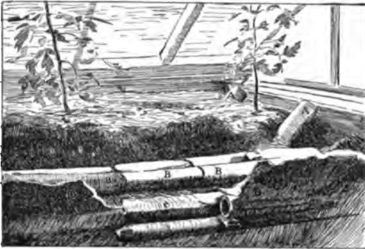
1183. Sub-irrigation with two tiers of tile.
