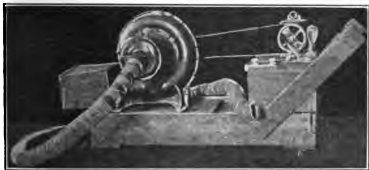
FIG. 122—Vacuum trap for storage insects.
