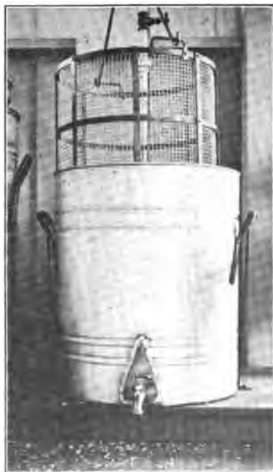
FIG. 54.—Blanching vat for vegetables. This is for a community size evaporator.
