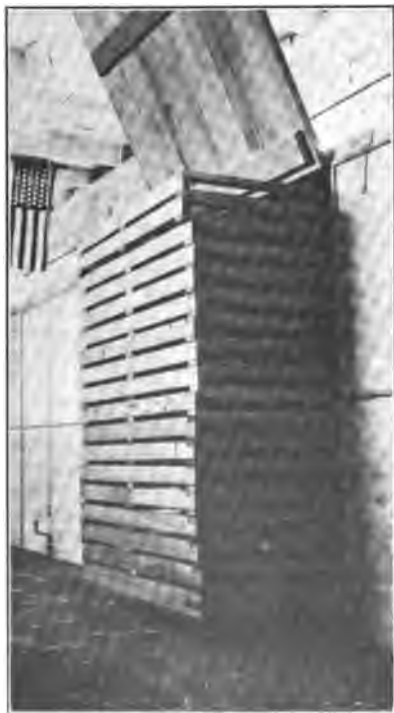
FIG. 51.—Community drying tunnel showing stack of trays ready for the dryer.
